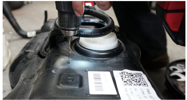
Drill pilot holes into the center of your marks. Be careful not to get plastic shavings into tank.
