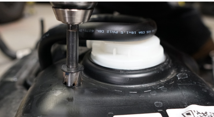
Drill holes out to 3/4". Be careful not to get any debris into the fuel tank.
