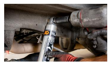
Install new shocks starting with the top bolt.
