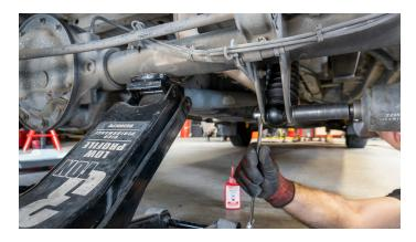
Use a jack to help you line up the lower shock mount holes on the axle with the shock. Apply threadlocker and install lower shock hardware.
