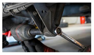
Remove old shocks starting with the lower bolt. Discard the shocks. Save factory hardware, you'll reuse it.
