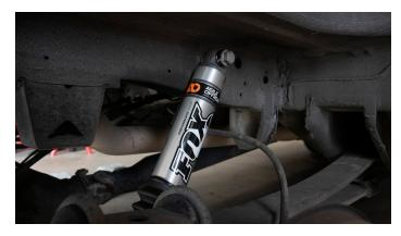
Torque upper shock bolt to 110 ft-lbs. Torque lower shock bolt to 75 ft-lbs. Reinstall wheels & torque lugs to 140 ft-lbs.
