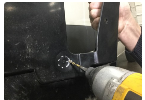
location for anchor screw
