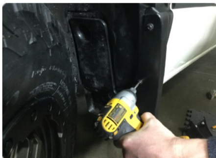
install T-25 screws
