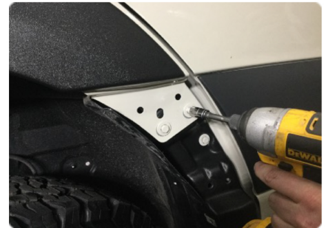
install fender bolts
