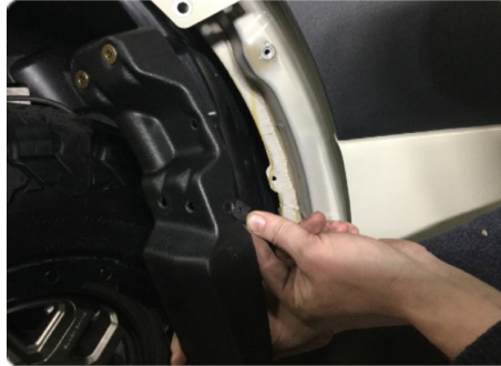
install speed nut
