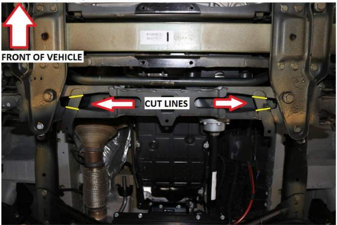
6) The main 401001-02 aluminum skid plate attaches to the vehicle via the factory holes noted in the image below. Take note of which holes will be utilized.
