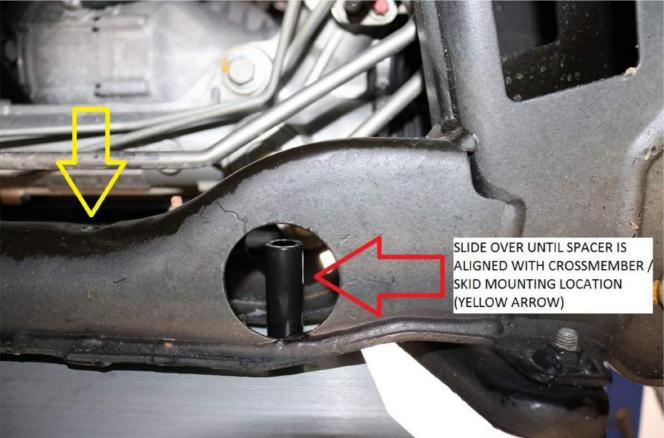
10) Install the  $3/8-16 \times 3.5$ " long carriage bolts through the spacer. Use a washer under the nylock nut. Just start the nut. Do not tighten at this time. See image below.
