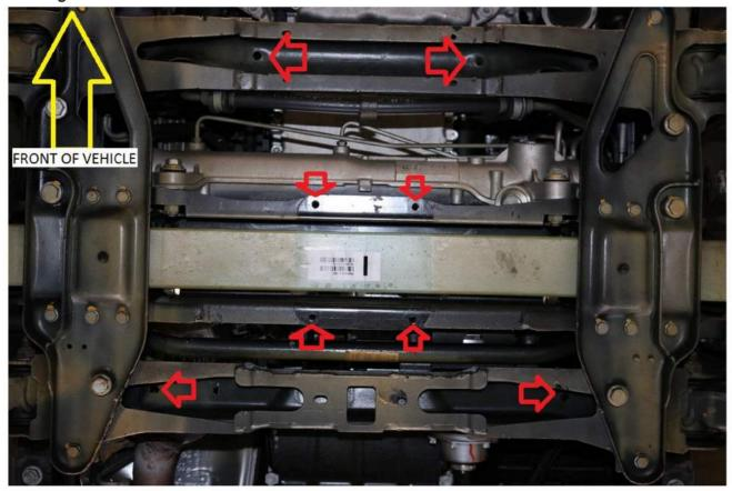
7) Raise the main aluminum skid plate into position. Try not to cover any of the mounting holes when raising it in place. Use a floor jack to lift into position.
