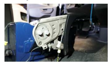
Remove parking brake cover and remove two bolts attaching the brake handle to the seat base. Save this hardware, you will reuse it.
