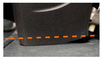
Trim the parking brake cover along the dotted line to ensure it doesn't interfere with the floor during operation.
