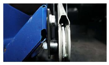
Bolt the parking brake handle to the relocation bracket using supplied hardware as shown. Sandwich the supplied spacers between the brake handle & relocation bracket.
