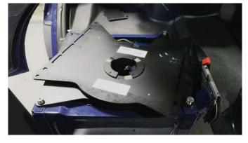
Route all electrical connections through the center hole to prevent them from being pinched during operation. Re-install the driver seat, tighten seat bracket bolts, and reconnect seat electrical connectors. Test swivel operation. Reconnect main battery. Congratulations, your installation is complete!
