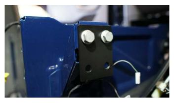
Bolt the supplied relocation bracket to the seat base as shown.
