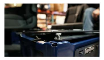
Place swivel onto seat base. Be sure to get all 4 bolts started before tightenen swivel onto the base.
