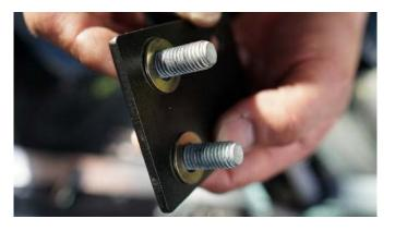
Use TWO washers on EACH factory parking brake bolt. Both washers should be on the side facing toward the seat base.
