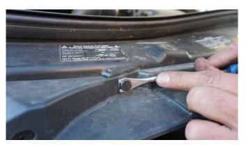
Use a plastic pin removal tool to remove the remaining push pins along the top edge.
