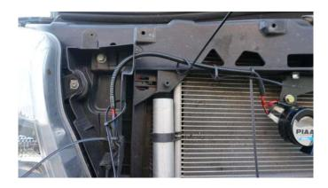
Drill several 1/4" holes along the edges of the shroud and a single 1/2" hole in the upper left corner. Route wiring and secure with zip-ties as shown.
