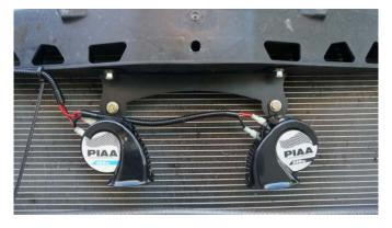
Mount horns to bracket using included hardware and attach the pre-assembled wiring harness to horns. Assemble as shown.
