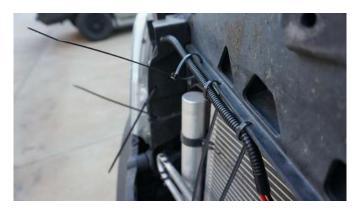
Drill several 1/4" holes along the edges of the shroud and a single 1/2" hole in the upper left corner. Route wiring and secure with zip-ties as shown.
