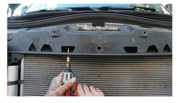
Drill 2 3/8" holes into the upper radiator shroud. Center the holes in the front openings as shown.
