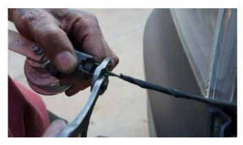
Cut factory horn wiring as close to the connector as possible and remove factory horn.
