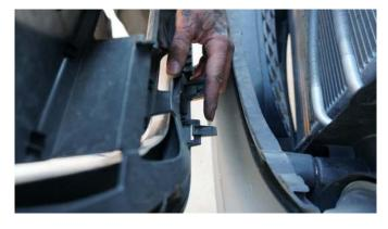
Depress tabs along the lower edge of the grill and pull firmly to remove it.
