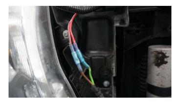
Crimp new wiring harness to factory horn wiring using included butt connectors. Attach red wire to green & black wire to brown. Once connected, apply heat from a heat gun or small torch to the connectors to activate the shrink wrap to ensure a weather-resistant seal.
