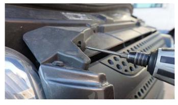
Loosen 2 T-25 Torx bolts at the top corners of the front grill.
