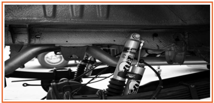
Install new shocks. Start with top bolt. Included washer goes between the shock & frame. Upper Shock Bolt Torque Specs: 110 LB (Note: clean factory bolts & apply loc-tite before installing)
