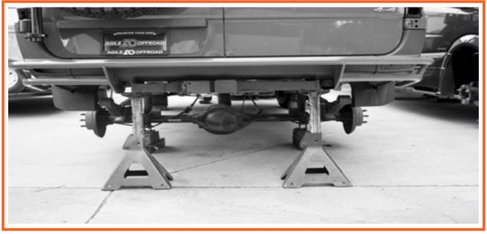
Lift vehicle and support vehicle with jack stands using trailer hitch or factory jack points. Remove wheels.
