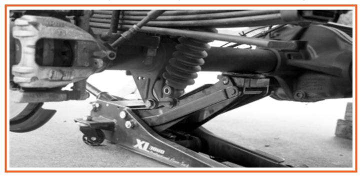
Use a jack to manipulate axle up or down to line up holes for lower shock bolt. Install lower shock bolt. Lower Shock Bolt Torque Specs: 75 LB
