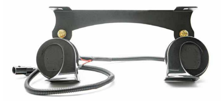
5. Hold the horn bracket against the upper radiator support assembly. Use a pencil to mark the bracket's mounting holes.
