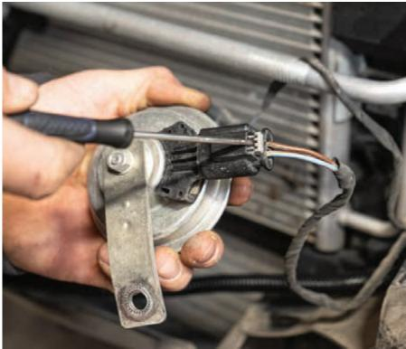
8. Plug the AO Horn Upgrade Harness into the factory horn wiring.
