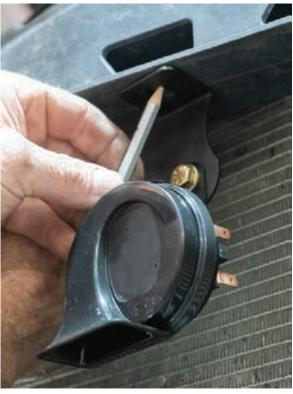
6. Use a 3/8 in. Drill Bit to drill through the previously marked points. Use the supplied hardware to mount the assembled bracket to the radiator support assembly.
