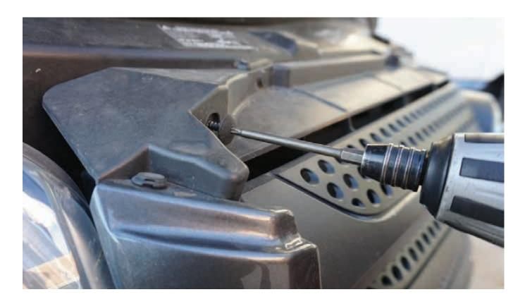
2. Use a Plastic Clip Removal Tool to remove the 4 remaining push pins along the top edge of the grill.
