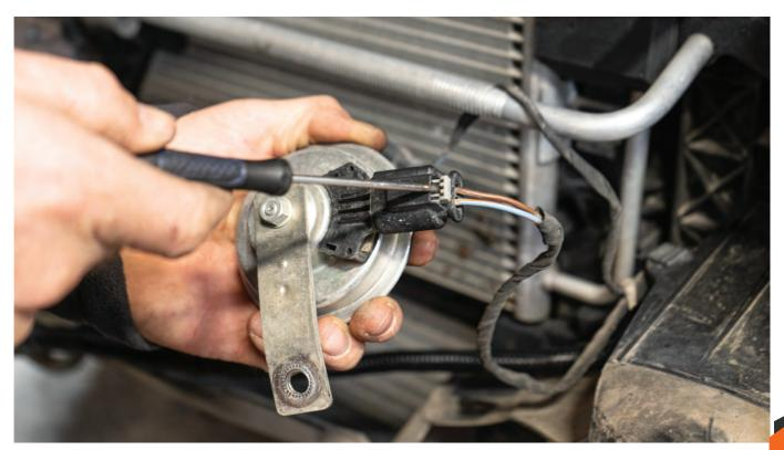
5. Mount the horns to the bracket using included hardware and attach the pre-assembled wiring harness to the horns.
