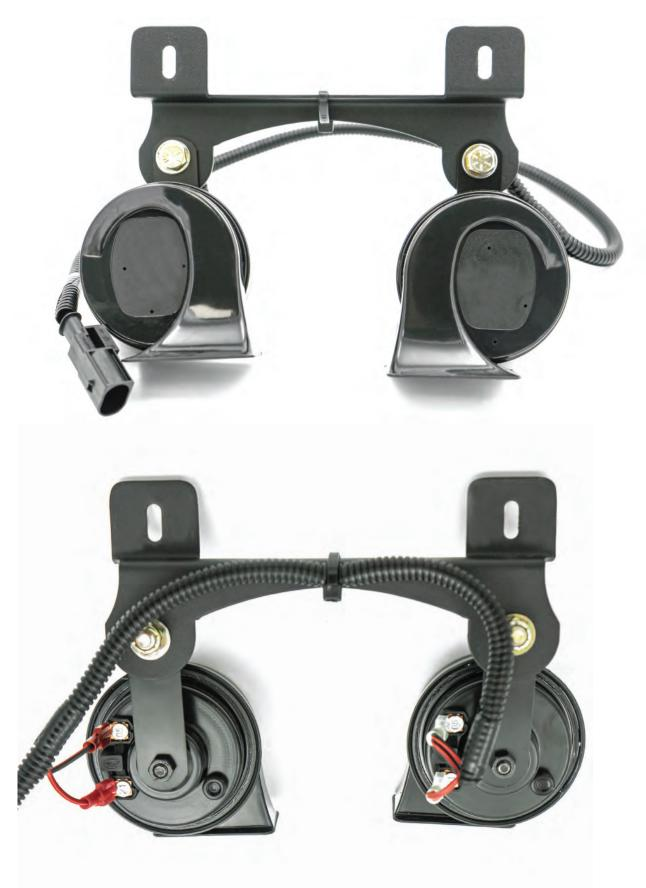
6. Mount horn bracket behind cruise control distance sensor bracket and re-assemble with previously removed T-25 Torx screws.
