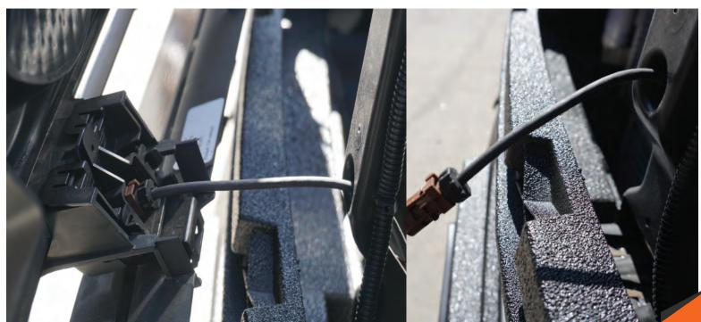
3. Remove the 2 T-25 Torx screws holding the "t-shaped" cruise control distance sensor brackets.
