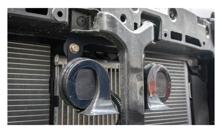
7. Plug the AO Horn Upgrade Harness into the factory horn wiring.
