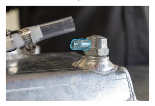
2. Use supplied 3/8 in. plastic T-fittings and (2) 3/8 in. x 2 in. clear tubes and route vent tube as shown below. Use tape (not supplied) to position the vent tubing away from the mounting holes and fuel sender.
