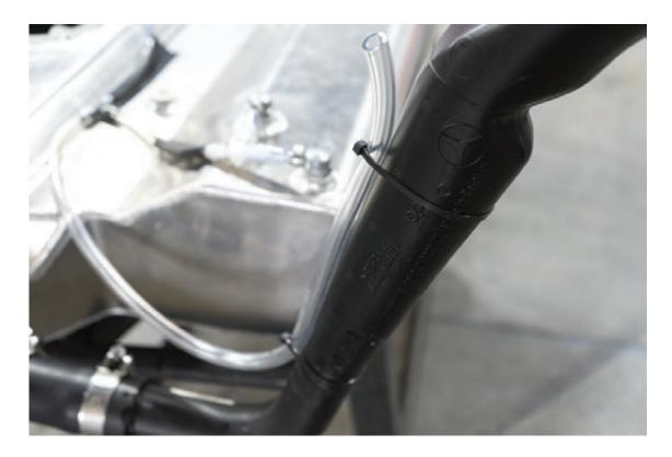
4. The final vent tubing assembly and routing is shown below. All vent tubing is clear. Color is for reference only.
