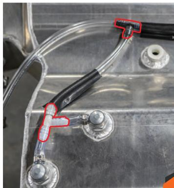
3. Use supplied zip ties to attach the open end of the vent tube to the fuel filler, as shown below.
