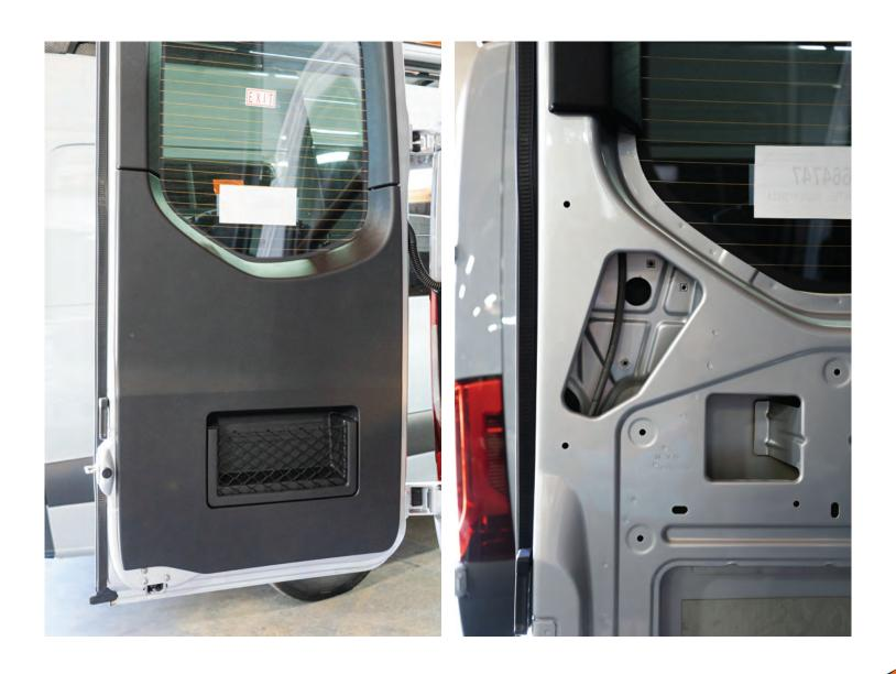
2. Mock the Rear Door Reinforcement Plate on the door, making sure that the preexisting door panel holes are not covered by the Plate. Use a marker and trace the Reinforcement Plate's (8) mounting points.
