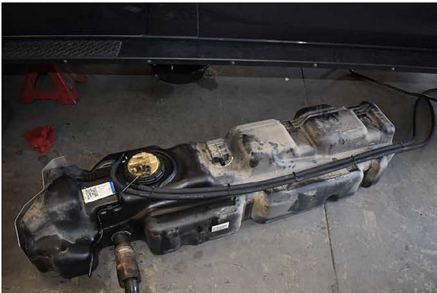
Attach assembled hoses and fittings to factory tank. Use zip ties to keep hose together and route as shown above.
