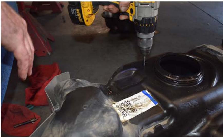
Drill a 1/8" pilot hole 1-1/4" from the threaded inlet. This will be for the filler line.
