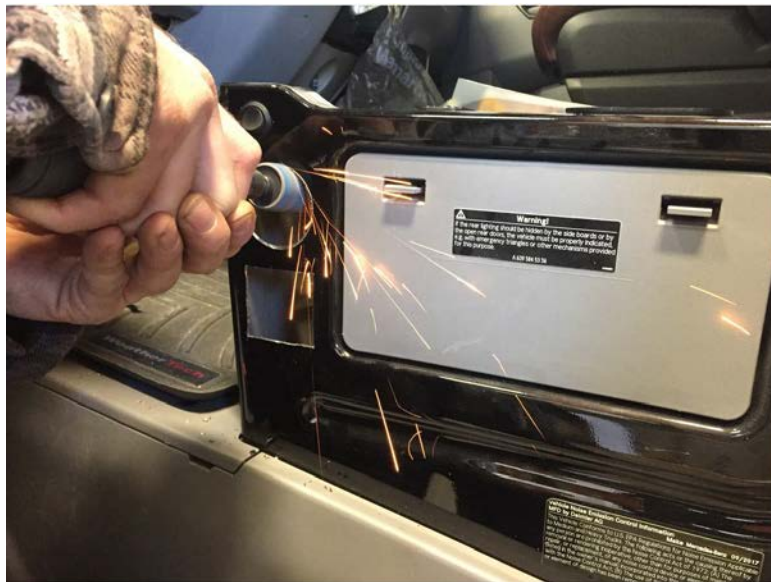
Above is an example of where you can install the auxiliary fuel gauge and switches. Locations may vary based on space.
