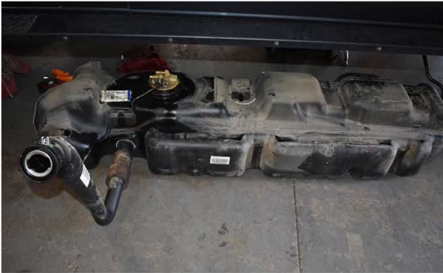
Remove factory fuel tank from vehicle.
