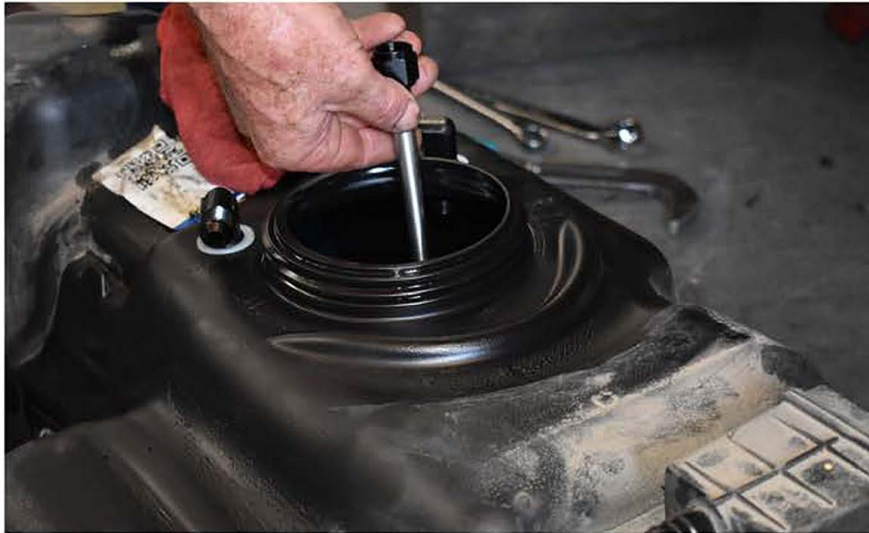
Install in-tank filler tube on to the fill side fitting.
