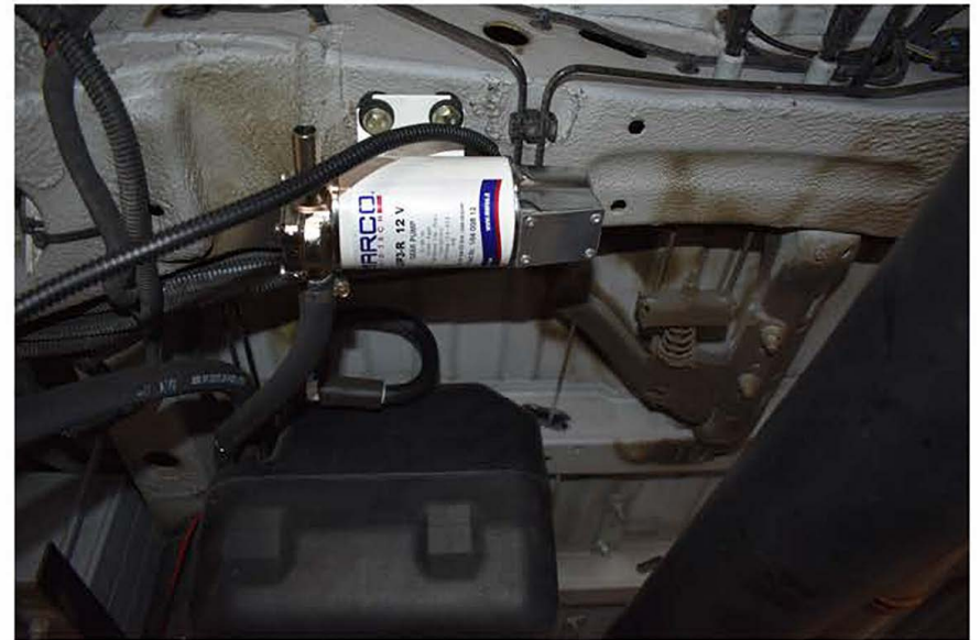
Attach supplied fuel pump to first crossmember behind the factory fuel tank. Mounting location can vary depending on available space.
