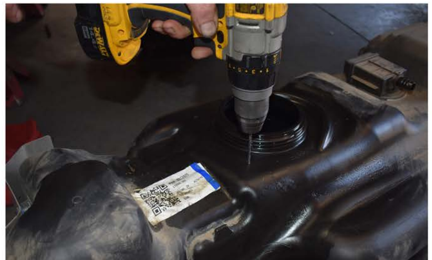
Drill a second 1/8" pilot hole 1-1/4" from the threaded inlet. This will be for the return line.
