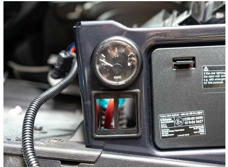
Above is an example of where you can install the auxiliary fuel gauge and switches. Locations may vary based on space.
