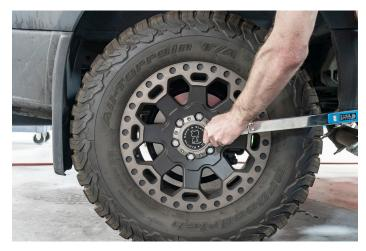
Re-install wheels using the appropriate lug nuts for the wheel. Lower vehicle on the ground. Torque the lug nuts to 125 ft-Lbs.
