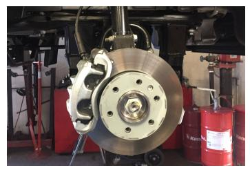
Lift your vehicle, support it with jack stands, and remove the wheels. Clean rotor flange & hub threads of rust and debris.
