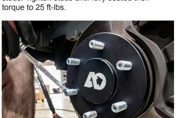
Apply a small amount of anti-seize to exposed wheel stud threads.
