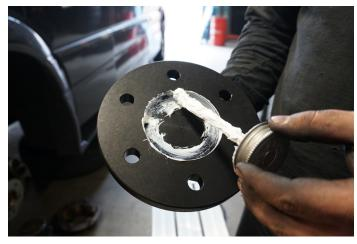
Apply a small amount of anti-seize to where the wheel spacer sits on the rotor flange. Install the Agile Wheel Spacer.
