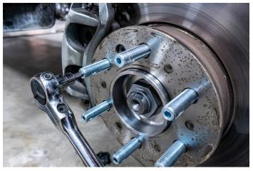
Use a 5/32" Allen key to tighten all of the wheel studs. Tighten studs until fully seated then torque to 25 ft-lbs.
